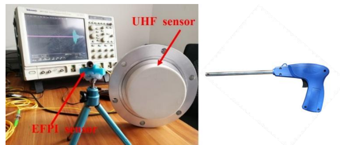
Picture 3: (a) The image of comparative test of EFPI sensor and UHF sensor, (b) The pulse discharge gun
