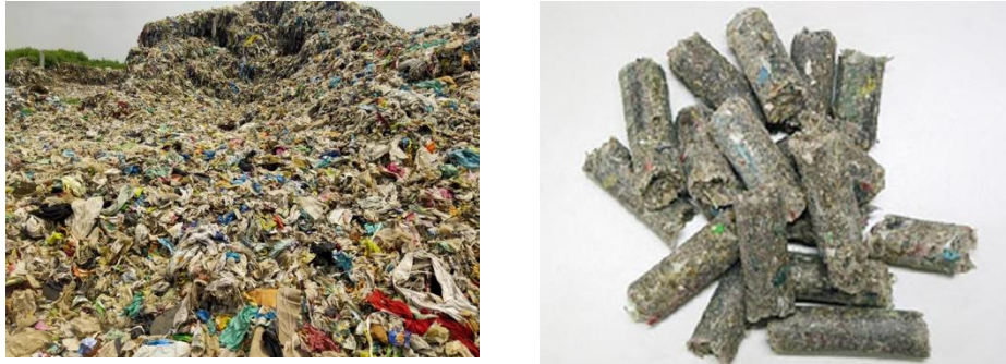
Picture 2: Physical Transformation from RDF-3 (Fluff) to RDF-5 (Briquettes).
