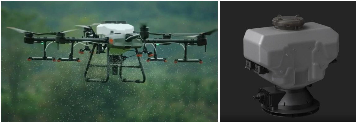
Picture 4: Attachment device for broadcasting system of agricultural drone
