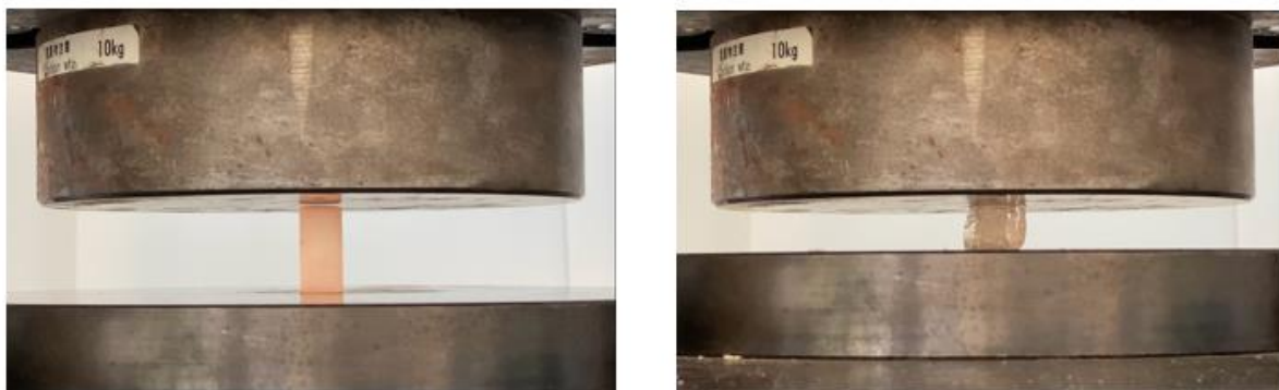
Picture 4: Specimen compressive before and after test
