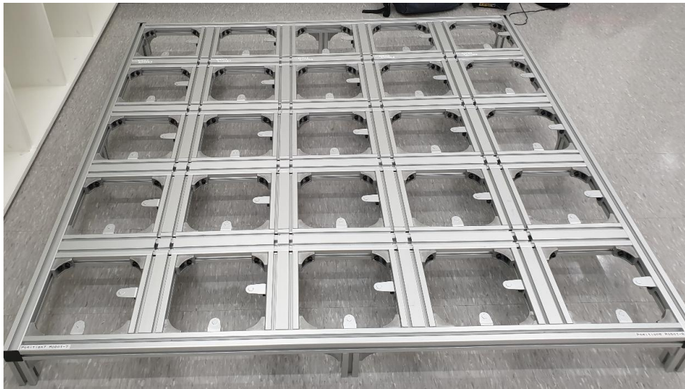
Figure 3: The design of grid rail for grid-based storage
